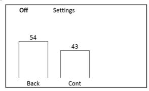
Use the first column up/down buttons to adjust the backlight to the desired level.
