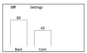
Use the second column up/down buttons to adjust the display contrast as required.
