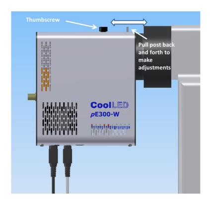
8.2 To make the adjustment, set up a typical sample on the microscope that gives an image over the whole field of view. Loosen the thumbscrew and slide the post back and forth until you achieve the maximum brightness with
