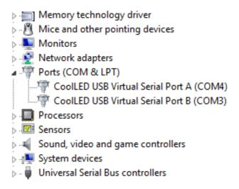
In this example the  $p\text{E-300}^{\text{white}}$  has been assigned two COM ports, COM3 and COM4. You may need this information to connect to the light source from your software control package. Either COM port may be used for control. Two COM ports have been assigned to allow for diagnostics to take place in parallel with communication and also allow for dual communication should that ever be desired.
