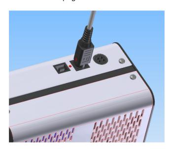
4.4 Connect the power connector from the DC power supply as shown. Ensure that the DC power supply is the one supplied with the product. Using non CoolLED power supplies may damage the light source and will invalidate the warranty. At this stage do not connect the mains power lead to the DC power supply.
