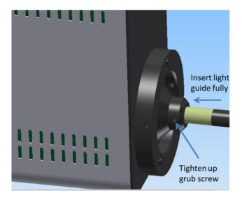
13.3 Do not bend the liquid light guides through sharp corners. It is recommended to ensure a minimum bend radius of 75mm. Ensure that the Light Source sits upright on a flat surface and keep the clearance of 200mm on both sides to ensure adequate airflow for the cooling system.
