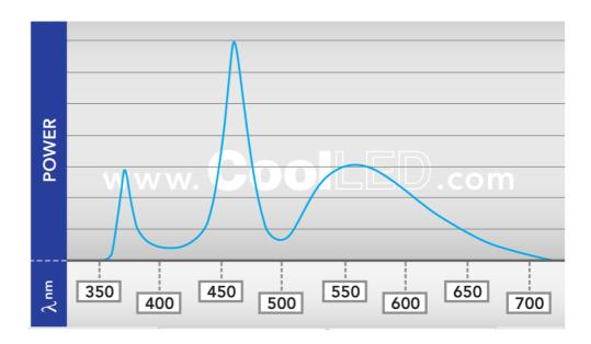
5.2 The  $pE-300^{\text{white}}$  has independent circuits giving the user control of the three main peaks of emissions. On the standard configuration, these are referred to as 1UV, 2B (blue) and 3GR (green, yellow, red).
