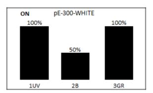
6.7 Individual bands can be switched off (de-selected) by pressing the 'select' button. Light is then only generated where it is required to excite the stains in use. This has many attractive benefits with improvements in contrast, cell viability and savings in energy.
